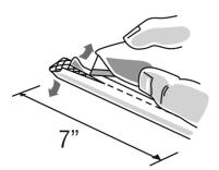
3. Push back Braid to loosen. Spread apart Braid as shown and bend the heating cable and work it through the opening in the Braid.
