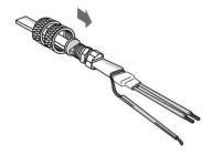
11. Install the strain relief in a Listed junction box. Ensure the sealing ring is compressed between strain relief body and junction box surface. Make connections using wire nuts provided and ensure the strain relief and lock nut are grounded. When installing into a non-metallic junction box, a UL-Listed bonding locknut shall be used and an additional conductor shall be provided to bond the locknut, cable braid and branch circuit ground conductor.
